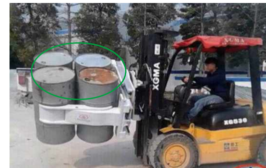
✓ 密封容器,人工手推车、叉车转运
